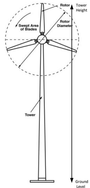
distance from grade to the top of the tower, plus the distance from the top of the tower to the highest point of the rotor's arc.
